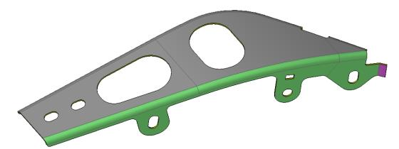
With this new functionality, the flange unfold operation can be done on the green area while leaving the purple area in its original position in order to obtain the following result.
